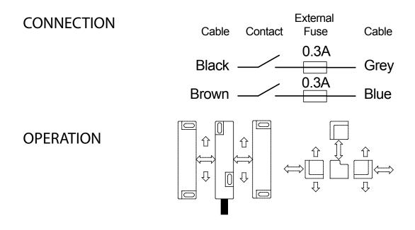
SWITCHING Face to Face 15mm ON 22mm OFF Side Min 7mm Max 22MM
