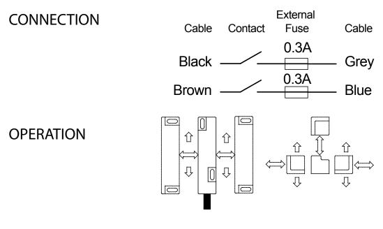
SWITCHING Face to Face 15mm ON 22mm OFF Side Min 7mm Max 22MM
